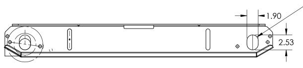
USE AN ANGLE GRINDER TO INCREASE OPENING FOR STEEL SPACER BUSHING ON BOTH SIDES
