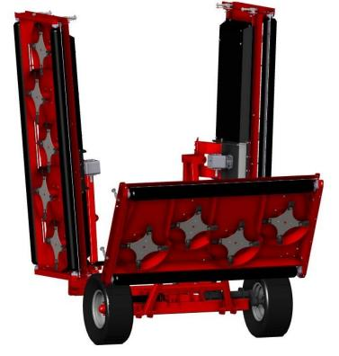
With *Pro-FORE* Progressive offers more blade options to optimize your cut to the growing conditions. Mounts in place of an existing Progressive one-piece or Pro-EZII blade without any modification to the existing blade spindle..
