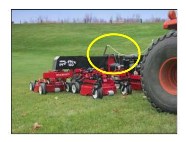
Progressive is pleased to announce that the AUTOMATIC WING CYLINDER LOCK VALVE (circled in the photo) can be added to an older Pro-Flex 120. Order update kit p/n 600600. This kit is suitable for any vintage of the Pro-Flex, however it does not add Pro Lift-N-Turn™ to a mower that is not already so equipped.
