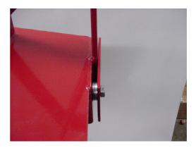
3. Mark the location of the second hole and drill the 17/32" mounting holes.
