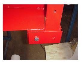
2. Align the plate up with the plate on the back of the mower. On the right hand side use the 4 – ½" washers as spacers to correct for the 3/8" flat bar.
