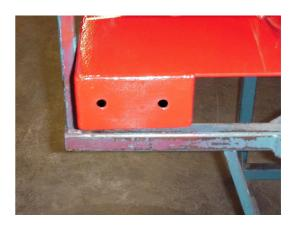
4. On the wing decks were the corner pin is located, mount the roller bracket in place using the  $\frac{1}{2}$ " x 1  $\frac{1}{2}$ " long bolt on the flat bar. The formed corner of the roller bracket must be on the outside, making it a right hand bracket.
