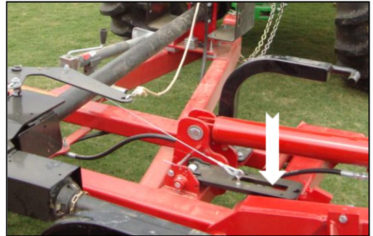
Each latch plate should lay flat against the wing frame when released. Ensure the center lock swivel is free to rotate.
