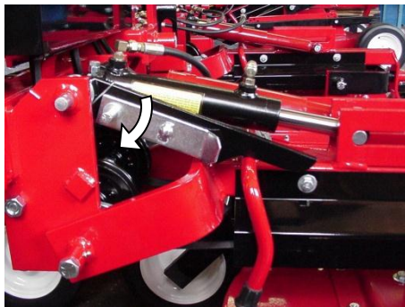
Mowing Position – Locks Disengaged
